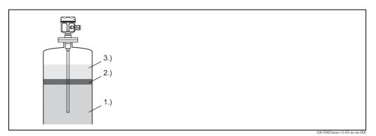
1.) Water, for example (the medium must be conductive  $\geq 100~\mu\text{S/cm}$ )
