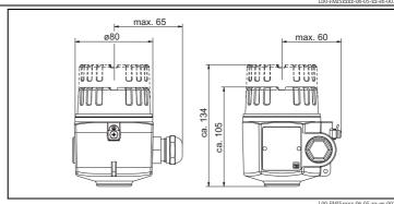
Aluminum housing F13 With gas-tight process seal
