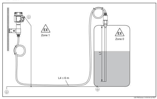
Rod length L1 max. 4 mRope length L1 max. 9.7 m (the maximum total length of L1 + L4 should not exceed 10 m).
