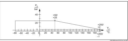
P<sub>n</sub>: Process pressure  $T_{D}$ : Process temperature
