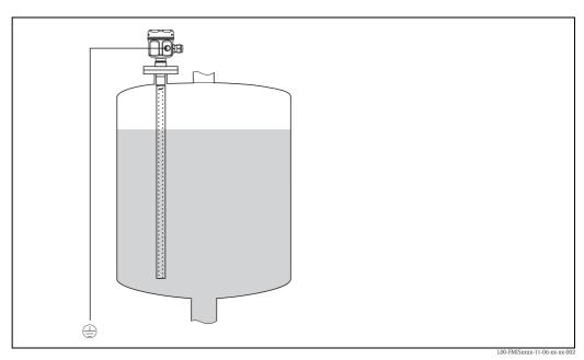
Probe with ground tube and grounding
