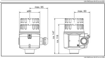
Aluminum housing T13 With separate connection compartment and gas-tight process seal
